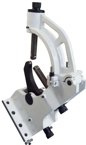
Manual Steady Rest Cutting range 240~400mm
